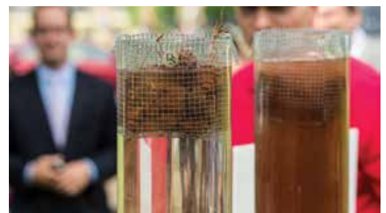
@USDA Slake test measuring aggregate stability.
